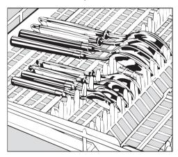
Spoons with thick handles may have to be placed as knives and forks with their heads in the holders.
